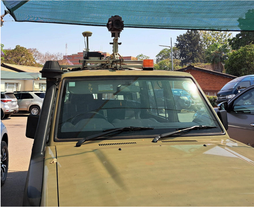
Figure 3: showcasing Road surface survey vehicle-mounted camera and GPS mapping antenna
