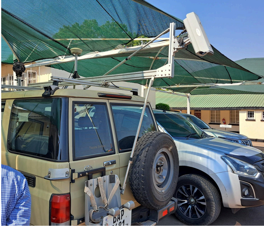
Figure 4: showcasing Road surface survey vehicle pavement camera
